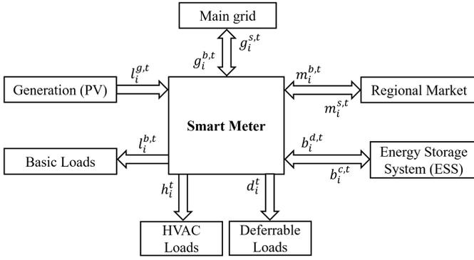
Fig. 2. An example of a Prosumer. The Prosumer is connected to the main grid on one hand and to the regional market on the other hand. Each Prosumer has an installed PV generator, an ESS, basic loads, HVAC and deferrable loads. The electricity flow is controlled by a smart meter.
