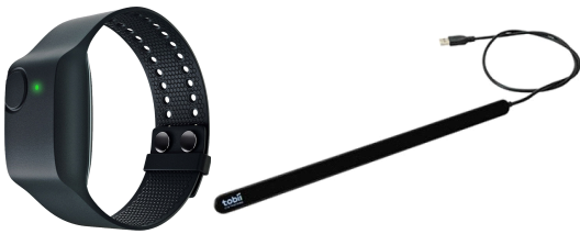
그림 1. 실험 측정장비. E4 Wristband(좌측), Tobii EyeTracker 4C(우측) Fig. 1. Experiment measurement device. E4 Wristband (left), Tobii EyeTracker 4C (right)
